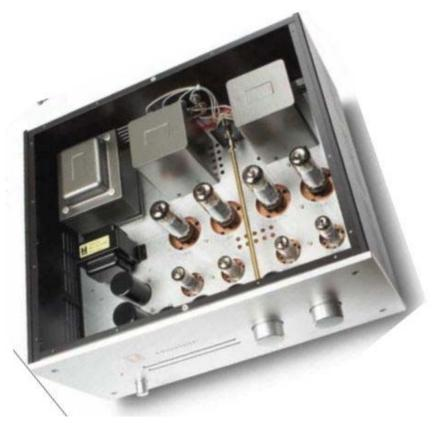
Overture ain't a Class A single-ended amplifier with a fancy triode tube as its bigger sister. Instead it's a common Class AB push-pull design with common EL-34 pentodes. What's the secret then?
